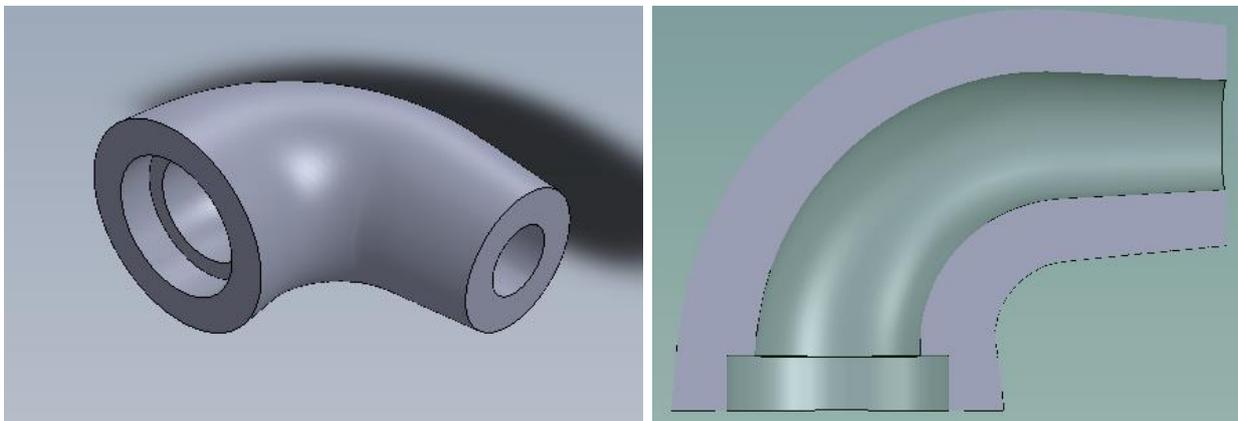
Figure 1: Isometric view (left) and cross section of the ceramic item
