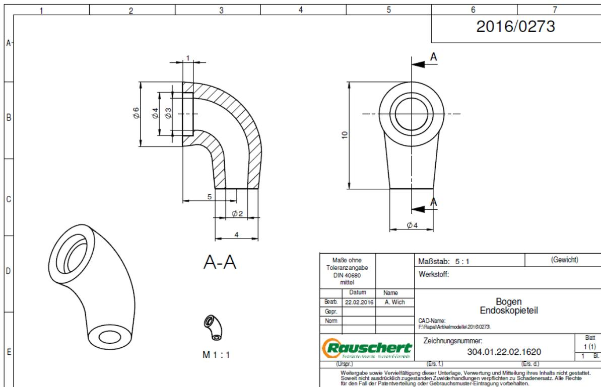
Figure 2: Technical drawing of the ceramic item for medical applications
