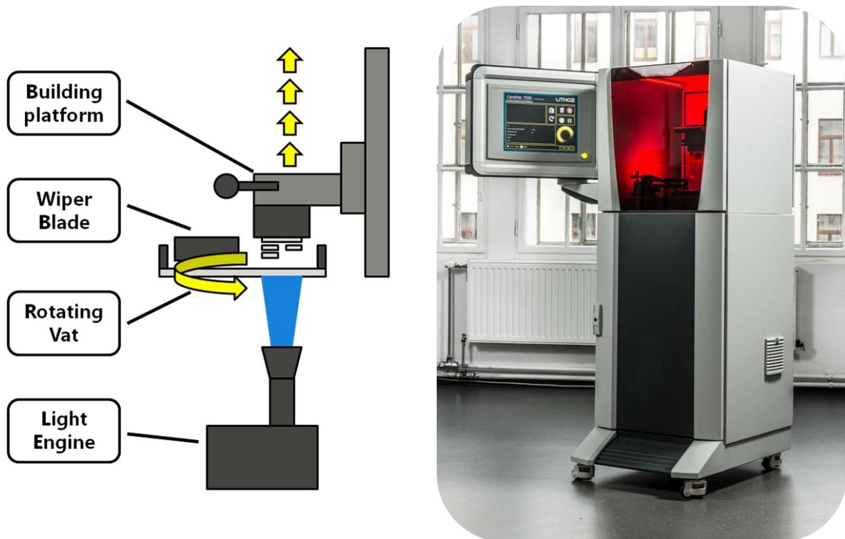
**Figure 3:** Schematic of the working principle of the CeraFab 7500 (left) and the actual printer (right)
